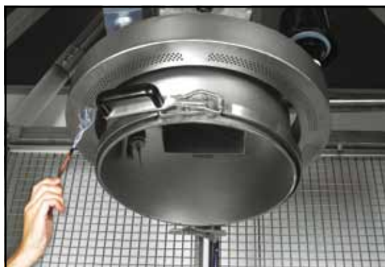
Screw Conveyor: Bin Suction Ring
