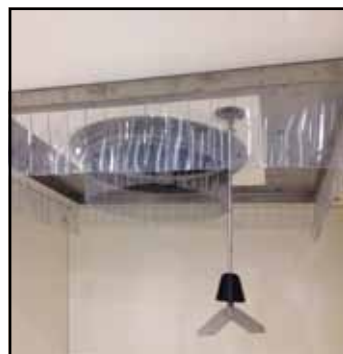
Bin Suction Ring & Max Level Sensor
